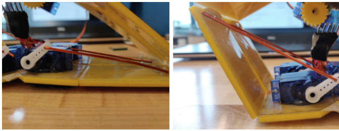
Fig. 6. Vertical expansion using a four bar linkage. Both the collapsed (left) and expanded (right) states are enabled by the pivot joint between the copper wire and the module elbow. Expansion is actuated via servos.
